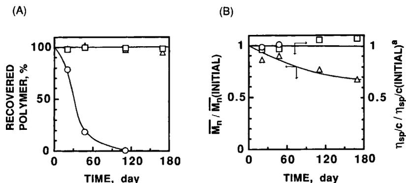
**Figure 1** Changes in (A) the weights and (B) the molecular weights of the films of the polyamides (4, 5, and 6) after the soil burial test (relative humidity, 80%, 27°C). The soil was composted for more than 10 years in the university farm (pH 7.5). Polyamide: (○) 4; (□) 5; (△) 6. (a) Viscosity number in 2,2,2-trifluoroethanol (1 g/100 mL, 25°C).
