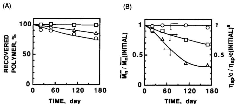
**Figure 5** Changes in (A) the weights and (B) the molecular weights of the films of the polyamides (4, 5, and 6) recovered after the soil burial test (relative humidity, 80%, 27°C). The soil has not been composted for more than 10 years in the university farm (pH 5.9).
