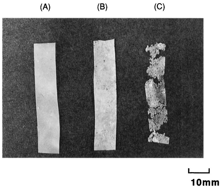
**Figure 2** Photographs of the films of polyamide 4 before and after the soil burial test as shown in Figure 1: (A) 0 days; (B) 21 days; (C) 48 days.
