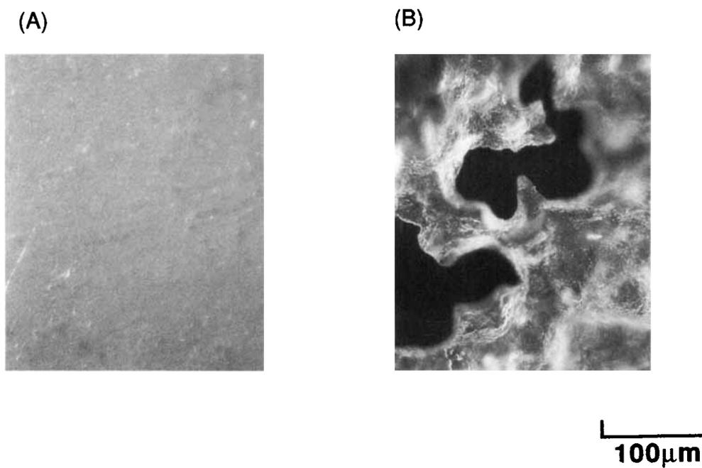
**Figure 3** Microscopic photographs of the films of polyamide 4 before and after the soil burial test as shown in Figure 1: (A) 0 days; (B) 48 days.
