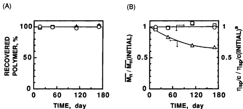
**Figure 4** Changes in (A) the weights and (B) the molecular weights of the films of the polyamides (4, 5, and 6) immersed in a phosphate buffer at 27°C.
